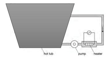
The hot tub system shown above has a volume of  $1.50~\text{m}^3$  and is filled with water at a temperature of 28.0~°C. The heater transfers thermal energy to the water at a rate of 2.70~kW while a pump circulates the water. Assume that no heat is transferred to the surroundings and  $1.00~\text{m}^3$  of water has a mass of  $1.00~\text{x}10^3\text{kg}$ .
